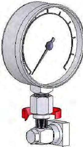
Figure 2. Connect Assembly to Test Port
