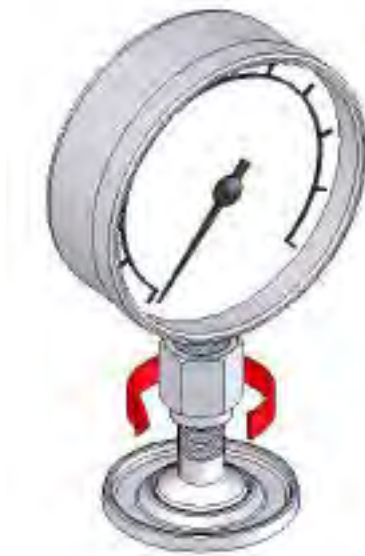
Figure 2-2. Connect Assembly to Test Port
