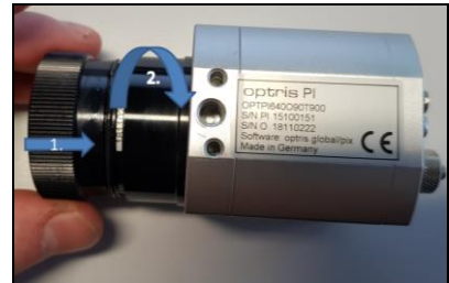
Figure 13: Inserting the lens
