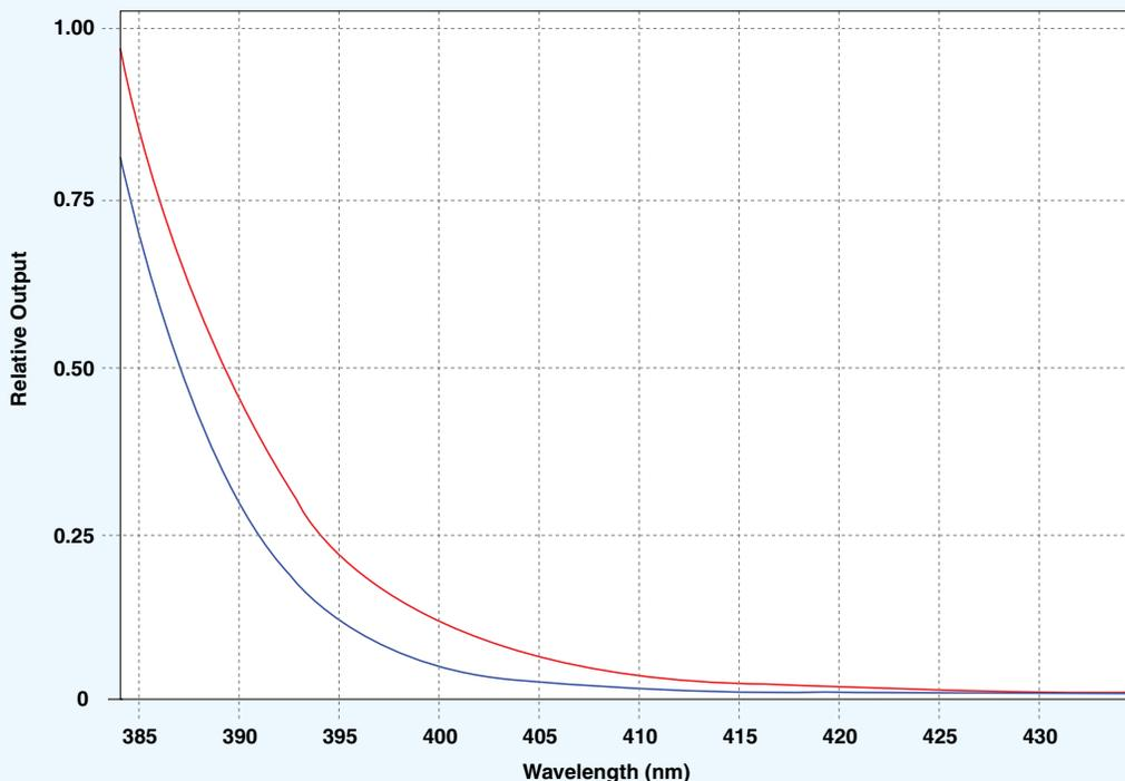
As the wavelength of the OPTI-LUX™ 365 moves into the visible light range, the black light filter significantly reduces the UV-A output of the lamp by as much as 50% at 400 nm.
