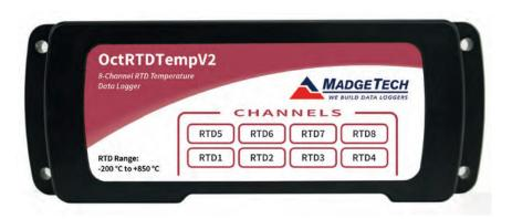
The OctRTDTempV2 is an 8-channel, RTD based temperature data logger with a reading rate of up to 4 Hz. It can measure and record up to 21,824 readings per channel. To maximize memory capacity, users can enable or disable channels. For easy identification, each channel can be named with up to a ten digit title. The storage medium is non-volatile solid state memory, providing maximum data security even if the battery becomes discharged. The OctRTDTempV2 makes data retrieval quick and easy.
