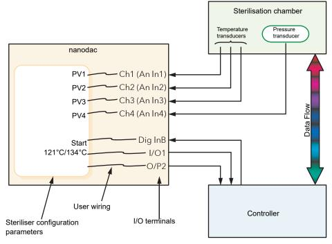
Figure 43 Typical steriliser application
