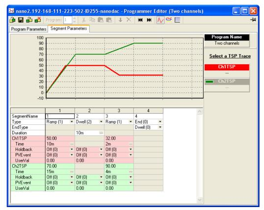
Figure 191 Two channel program display
