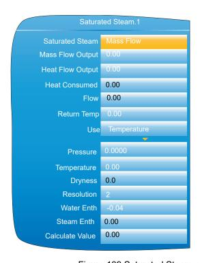
Figure 139 Saturated Steam configuration
