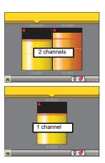
Figure 20 Vertical bargraph display mode
