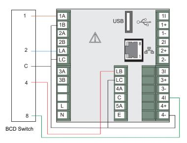
Figure 40 BCD Switch Physical Wiring
