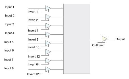
Figure 147 Logic (8 input) block schematic
