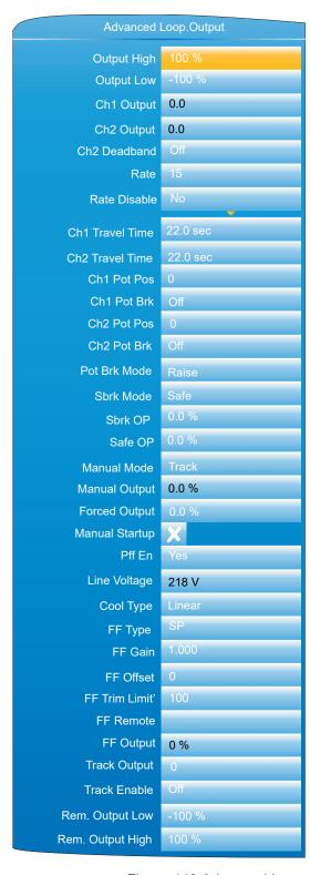
Figure 113 Advanced Loop Output menu
