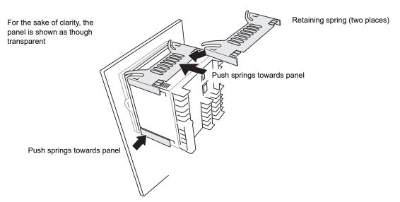
Figure 1 Securing the Instrument
