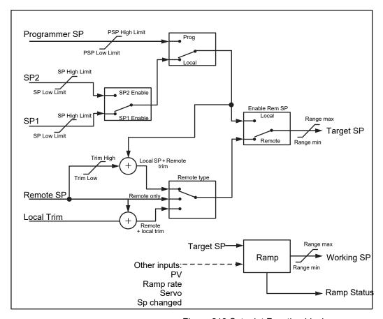
Figure 213 Setpoint Function block
