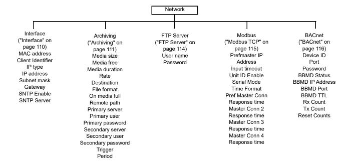
Configuration nanodac™ Recorder / Controller
