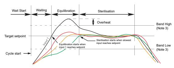
Figure 42 Steriliser cycle
