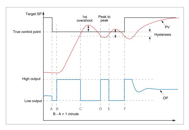
Figure 206 Autotune heat only process (from below SP)
