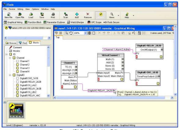
Figure 171 Graphical wiring Editor
