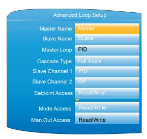
Figure 105 Advanced Loop Setup menu
