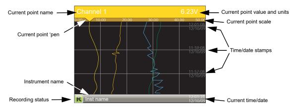
Figure 9 Typical display screen (Vertical trend)
