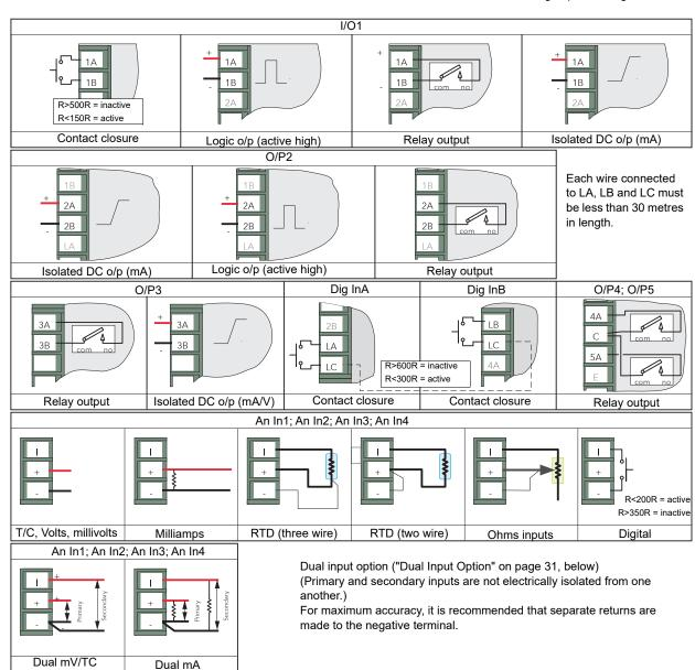
Figure 4 Connector locations and pinouts (rear panel)
