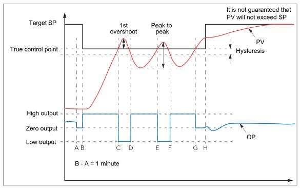
Figure 205 Autotune heat/cool process
