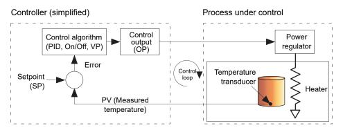
Figure 198 Control loop example
