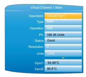
Figure 97 Maths channel configuration (typical)
