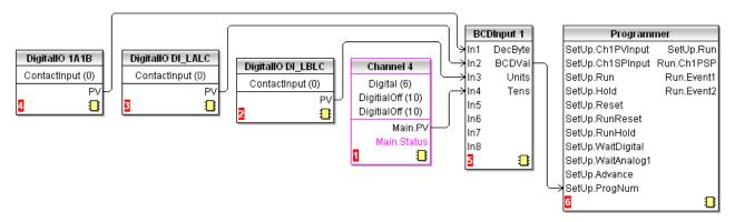
Figure 39 BCD Switch Wiring
