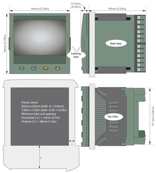
Figure 2 Mechanical installation details (standard case)
