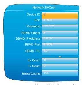
Figure 85 BACnet configuration menu
