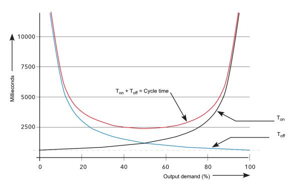
Figure 220 Time proportioning curves (Minimum on time = 625ms)
