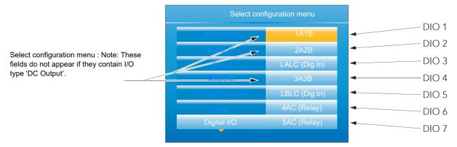
Figure 131 Digital I/O top level menu
