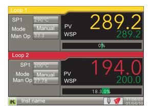
Figure 26 Loop displays
