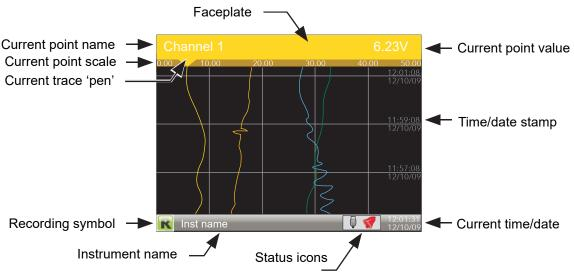
Figure 18 Vertical trend mode display elements
