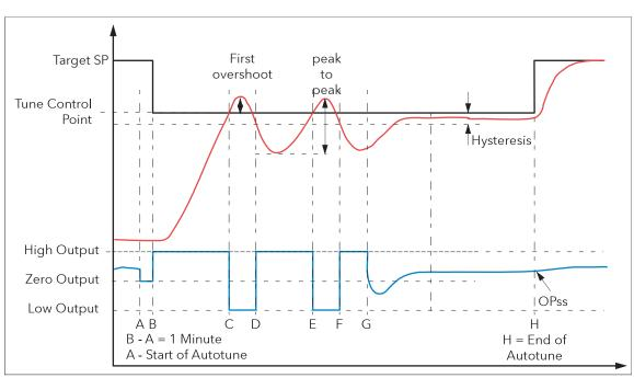
Figure 209 Autotune from below setpoint
