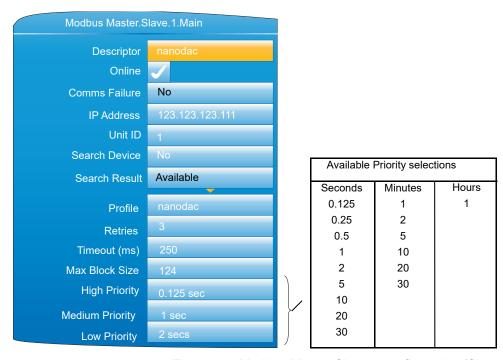
Figure 123 Modbus Master Slave 1 configuration (Slave 2 similar)
