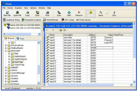
Figure 55 iTools display showing input tags.
