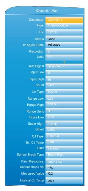
Figure 90 Channel main menu (expanded)
