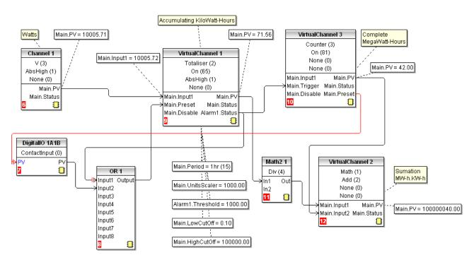
Figure 100 Linking a counter and totaliser
