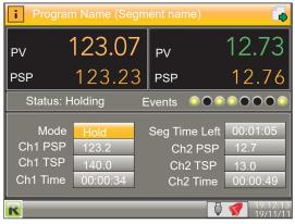
Figure 29 Two channel program in Hold mode
