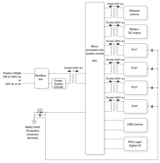
Figure 224 Isolation diagram
