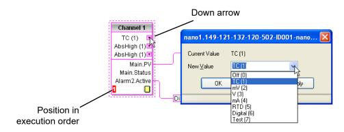
Figure 172 Function block example
