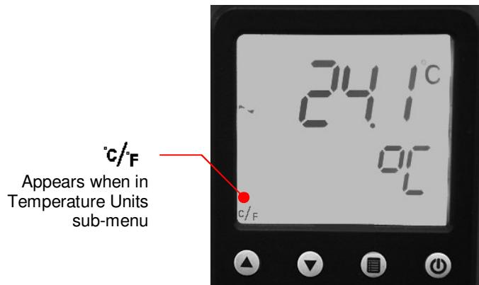
**To Access:** Press the key until the °C/°F appears on the display.
