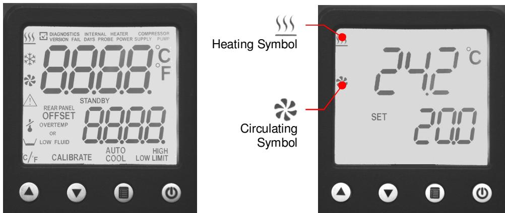
6. **Set the Safety Set temperature.** This is a "Do Not Exceed" temperature setting for your Circulator and is the temperature at which the heater will be turned OFF in the event that the liquid level in the bath drops too low or the Circulator malfunctions. It is normally set about 5° higher than the desired operating temperature. Setting the Safety Set temperature is a four-step process.
