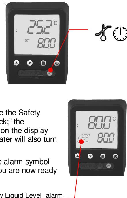
Over-Temperature/Low Liquid Level alarm
