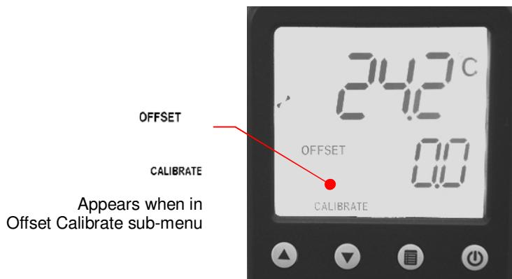
**To Access:** Press the
