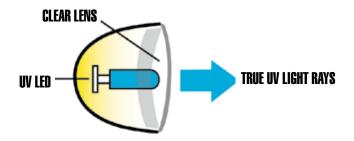
UV LEDs produce only true and efficient UV light. The CPS **UVPRO** provides UV-A (Long wave UV) 325-375nm. Instant on LED provides the fastest leak inspection of any light available.
