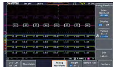
Display analog waveform converted from digital signal
