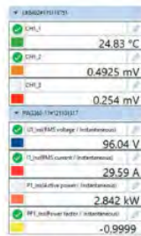
Monitor display (up to 512 parameters)
