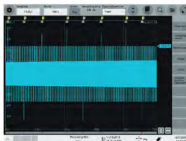
Continuous acquisition with no blind time
