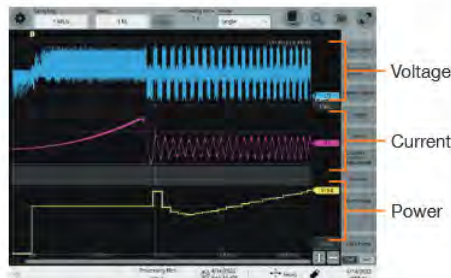
Example display of power calculation results
