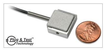
Series R04 smart sensors are designed for tension and compression measurement applications with tight space constraints. These extremely compact force sensors feature threaded holes on two sides, which can accept a variety of hooks and implements. Capacities available from 0.25 to 100 lbF [1 to 500 N]. Compatible with Mark-10 indicators (sold separately) through unique Plug & Test<sup>TM</sup> technology.
