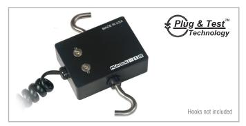
Series R03 smart sensors are designed for tension and compression measurement applications in virtually every industry. Threaded holes on two sides can accept a variety of hooks and implements, making this sensor particularly well suited for inline tests. Capacities available from 0.25 to 100 lbF [1 to 500 N]. Compatible with Mark-10 model 5i and 3i indicators (sold separately) through unique Plug & Test™ technology.
