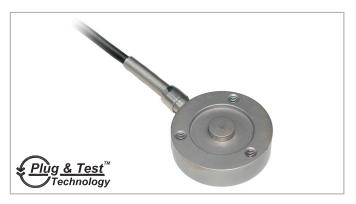
Series R02 button type smart sensors are designed for compression measurement applications in virtually every industry. Compact and rugged, Series R02 sensors are ideal for heavy duty applications with space constraints. Capacities available from 100 to 10,000 lbF [500 N to 50 kN]. Compatible with Mark-10 model 5i and 3i indicators (sold separately) through unique Plug & Test<sup>TM</sup> technology.
