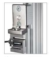
AC1018 Test stand mounting kit Adapts a Series R01 sensor to most test stands (except ESM303, ESM303H, ESM1500, ESM1500S, ESM750S, & TSB100)
