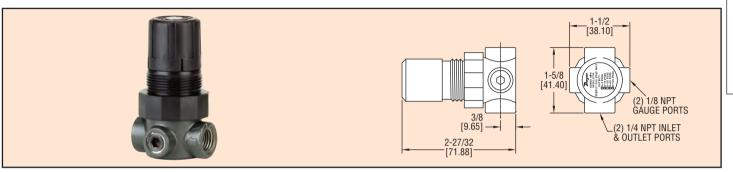
The Series MPR Miniature Pressure Regulators are compact units that provide low cost, high performance pressure regulation of compressed air or air/water. The low torque, non-rising adjustment knob with locking capability provides easy and precise adjustment. Models for use with air are self relieving. Models for air/water are non-relieving.
