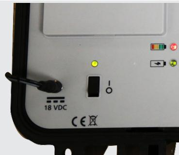
**Step 1:** Turn ON the MGFL100 transmitter and allow it to boot up.
