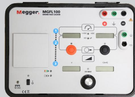
Connect the red terminal to the IT Filter box input.
