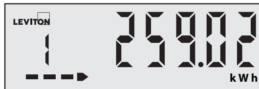
Figure 7 - LCD Appearance in Proper Operation (Example)
