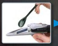
1 Apply 1-2 drops onto the prism.
