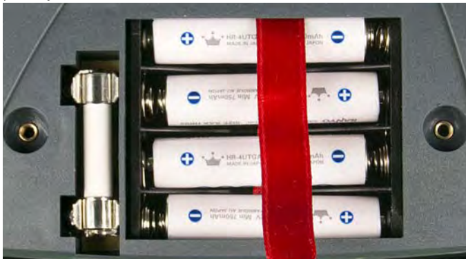
Figure 6.1: Correct Battery Polarity
