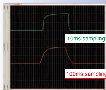
Measurement comparison of abrupt load change in waveform with 10 ms (upper trace) and 100 ms sampling
