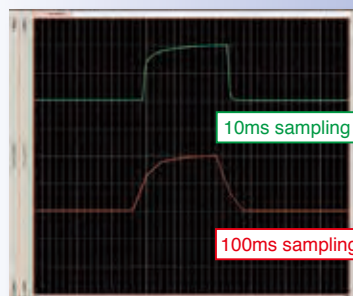
Measurement comparison of abrupt load change in waveform with 10 ms (upper trace) and 100 ms sampling
