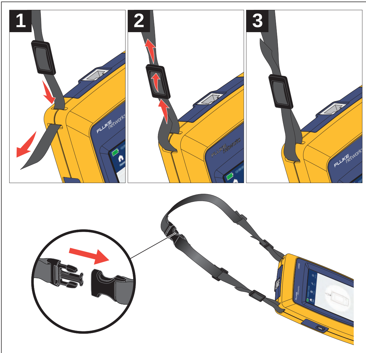
Figure 1. Hang Strap Attachment
