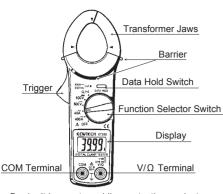
Barrier:It is a part providing protection against electrical shock and ensuring the minimum required air and creepage distances.
