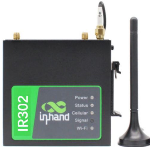
Chuck Antenna Installation
