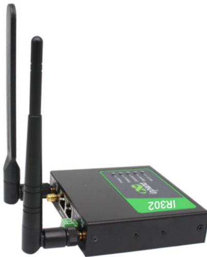
Glue Stick Antenna Installation
