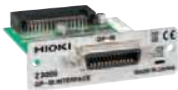
GP-IB INTERFACE Z3000
