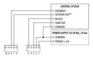
Wiring for models with RTD/thermistor:
