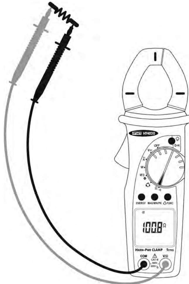
Fig. 7: Use of instrument for resistance and continuity test
