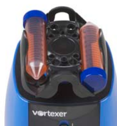
50 mL conical tubes x 2 (horizontally mounted)
