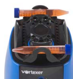
15 mL conical tubes x 2 (horizontally mounted)
