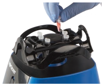
0.5 mL microfuge tubes x 6 (vertically mounted)
