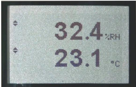
The LC display of the HP21 has a backlight which can be set to be on all the time or whenever a key is pressed. The backlight can also be disabled.
