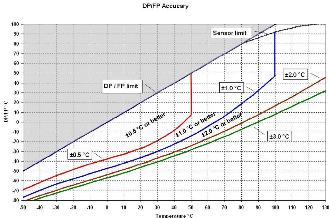
**Example:** at a temperature of 20 °C, a dew point value of -37 °C is measured with an accuracy of ± 1.0 °C or better.
