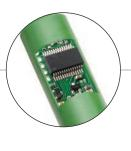
Stored pH calibration information includes: calibrated buffers, date, time, offset and slope characteristics of the electrode. Conductivity calibration information includes: calibrated conductivity standards, date, time, and cell constant of the sensor. Dissolved oxygen calibration information includes: standards used for calibration, date, time, altitude and salinity correction.
