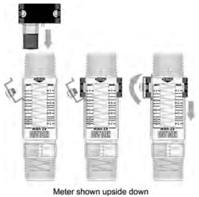
Figure 12: Vibration locking kit installation
