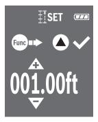
Press the measure button **2** [ $\blacktriangle$ ] to go to the stake out measurement display. Press the measure button **2** [ $\blacktriangle$ ] again to start the stake out measurement function. Move the laser measure slowly from the starting point.
