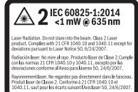
and do not stare into the laser beam yourself. This laser measure produces class 2 laser radiation and complies with 21 CFR 1040.10 and 1040.11 except for deviations pursuant to Laser Notice No. 50, dated June 24, 2007. This can lead to persons being blinded.
