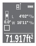
Aim and press the measure button 2 [▲] again to take the measurement for length which will appear on the top line of the measured-value lines d.
