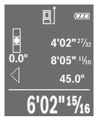
Press the measure button **2** [**\Lambda**] to activate the laser. Make sure the measuring reference point remains stable. Press the measure button **2** [**\Lambda**] to take the first measurement **A**. Press the measure button **2** [**\Lambda**] to take the second measurement **B**.
