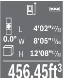
Aim and press the measure button **2** [**A**] again to take the measurement for length which will appear on the top line of the measured-value lines **d**.
