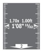
The laser measure continuously measures the distance to the starting point. The defined length and actual measuring value are shown in the display. The large arrows that display at the top or bottom of the screen indicate the positions of the previous or next pre-set measurement. For example, if the bottom arrow shows the
