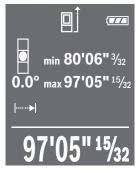
Watch the numbers move in real time in result line **e** as you move the laser measure towards or away from the object you are aiming at.
