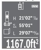
Place the laser measure on the floor and aim the laser at the ceiling, then press the measure button 2 [ $\blacktriangle$ ] to measure the room height H. The measured value is displayed in the top measured-value line d. The laser remains active.
