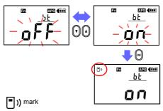
Lights up: Wireless communication function is on. Lights off: Wireless communication function is off. Flashes: Performing wireless communication
