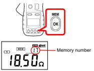
When the number of values saved in the instrument's memory reaches 2,000, the display will show "FULL," and you will not be able to save additional values. Delete unneeded values to free up space.
