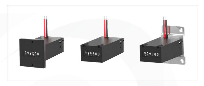
The 4916 Series incorporates the latest manufacturing technology together with basic design to achieve high performance over a wide temperature range with low power consumption. These counters can be mounted by two front flange styles, base mount or behind the panel (front mount). The 4916 has UL approvals and can operate over a wide voltage range of DC or AC power.
