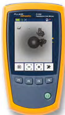
FI-500 displaying a dirty fiber endface
