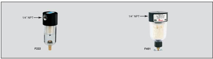
Compressed air filters protect equipment and instrumentation from harmful contaminant's such as dirt, water and oil. Liquids are continuously coalesced and released through the manual drain valves. Replaceable filter element removes particles and droplets as small as 0.01 micron with 93% efficiency. Units have 1/4" female NPT inlet and outlet and manual drain valve.
