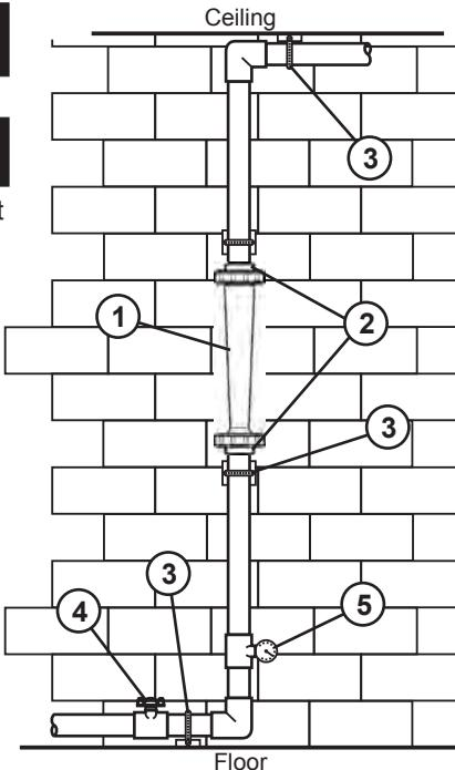
**3. Wall, floor and ceiling mounts and supports are to be carefully aligned and sturdy. Wall, floor and ceiling supports are recommended as needed. This is to maintain pipe alignment and to prevent vibration.**
