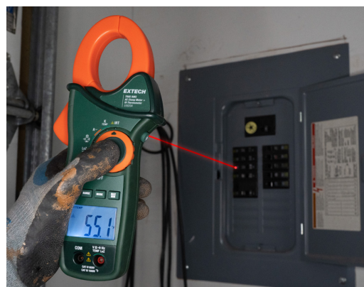
Built-in IR thermometer with laser pointer for locating hot spots and overheating motors.
