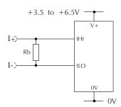
Measuring a current from a circuit which is floating with respect to the meter's supply, i.e. the current and the meter's power supply are isolated from each other. Ensure jumper link J1 is fitted.
