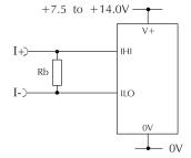
Measuring a current from a circuit which is floating with respect to the meter's supply, i.e. the current and the meter's power supply are isolated from each other.
