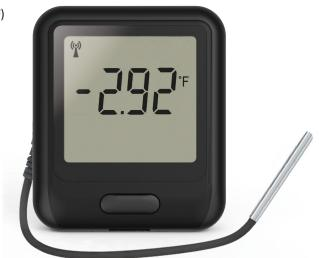
The sensor is IEEE 802.11b compliant, supports WEP, WPA/WPA2 encryption and enterprise networks.
