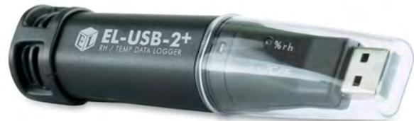
This standalone data logger measures and stores over 16,000 temperature and humidity readings from -35 to +80°C (-31 to +176°F) and 0 to 100%RH range at a resolution of 0.5°C (1°F) and 0.5%RH.
