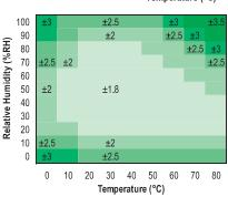
Typical accuracy of relative humidity measurements given in %RH for temperatures 0 to 80°C.
