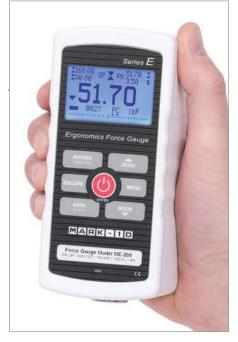
Series E push / pull force gauges make job task analysis and ergonomics analysis simple and accurate, ideal for workplace design, strength assessment, and ergonomic studies. Series E presents the ergonomist and other professionals with a simple and economical testing solution. 100 lbF, 200 lbF and 500 lbF (500, 2,500, and 5,000 N) capacity force gauges are available, along with a wide range of attachments for various applications.
