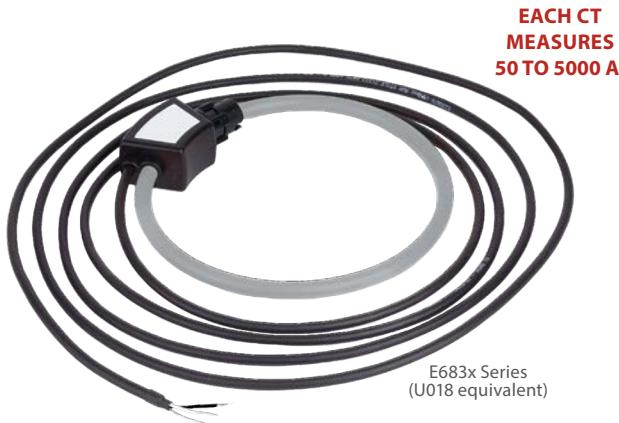
The E683x Series of Rogowski flexible rope style current transducers (CTs) provide secondary AC voltage proportional to the primary (sensed) current. For use with E5xxxA and E2x Series power meters, the E683x Series CTs provide a cost-effective means to transform electrical service amperages to a voltage compatible with monitoring equipment. The flexible core makes it easy to fit in tight enclosures.
