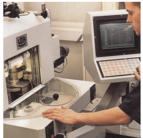
Figure 25.4 LEFT: Diamond turning machine; RIGHT: Lens polishing
