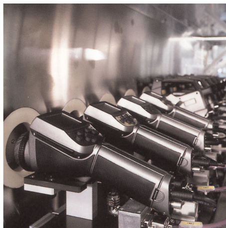
Figure 25.5 LEFT: Testing of infrared cameras in the climatic chamber; RIGHT: Robot used for camera testing and calibration
