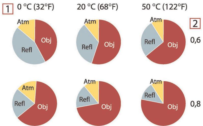
**Figure 17.3** Relative magnitudes of radiation sources under varying measurement conditions (LW camera). 1: Object temperature; 2: Emittance; Obj: Object radiation; Refl: Reflected radiation; Atm: atmosphere radiation. Fixed parameters:  $\tau = 0.88$ ;  $T_{\text{refl}} = 20^\circ\text{C}$  ( $+68^\circ\text{F}$ );  $T_{\text{atm}} = 20^\circ\text{C}$  ( $+68^\circ\text{F}$ ).
