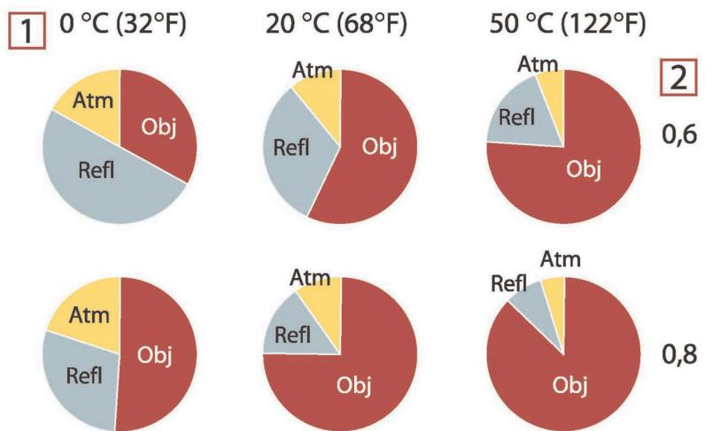
**Figure 17.2** Relative magnitudes of radiation sources under varying measurement conditions (SW camera). 1: Object temperature; 2: Emittance; Obj: Object radiation; Refl: Reflected radiation; Atm: atmosphere radiation. Fixed parameters:  $\tau = 0.88$ ;  $T_{\text{refl}} = 20^\circ\text{C}$  (+68°F);  $T_{\text{atm}} = 20^\circ\text{C}$  (+68°F).
