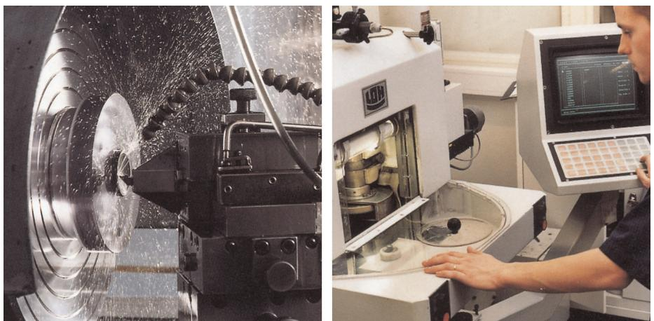
Figure 12.4 LEFT: Diamond turning machine; RIGHT: Lens polishing
