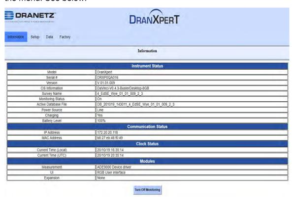
The Information page provides instrument status information, such as the serial number, firmware version, monitoring state, power source/battery charge status, IP address, and current time.
