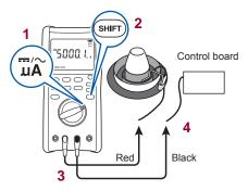
Example: Measuring the current of the burner flame (µA)
