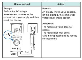
3 Check that the fuse is not broken.
