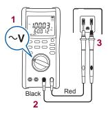
Measure the AC voltage. Measure the frequency simultaneously.
