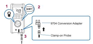
Set the clamp-on probe and the instrument to the same range.
