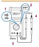
The open terminal voltage is approx. 2.5 V or less. The measurement current (DC) is approx. 96 nA. (p. 87) To avoid damage to the measurement object, check the specifications before use.
