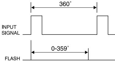
**NOTE:** If the input signal frequency exceeds upper or lower limits, the alarm dashes (----) will be displayed or the strobe will stop flashing.
