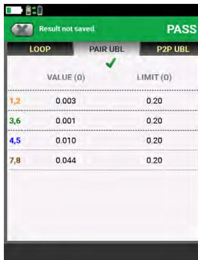
Too much unbalance causes saturation of the Power Sourcing Equipment transformer. This results in data distortion, causing bit errors, retransmits and even non-functional data links.
